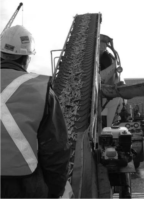
Used to install fibre reinforcing from the ground to the top of a concrete truck
