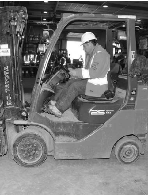
Used to transport and hoist equipment and materials around a jobsite
