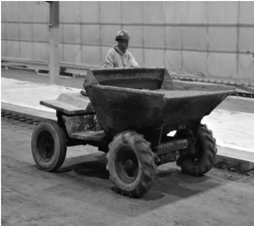
Used to transport fresh concrete from the concrete truck to the point of deposit
