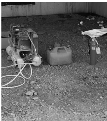
Used to power impact tools and other equipment powered by compressed air
