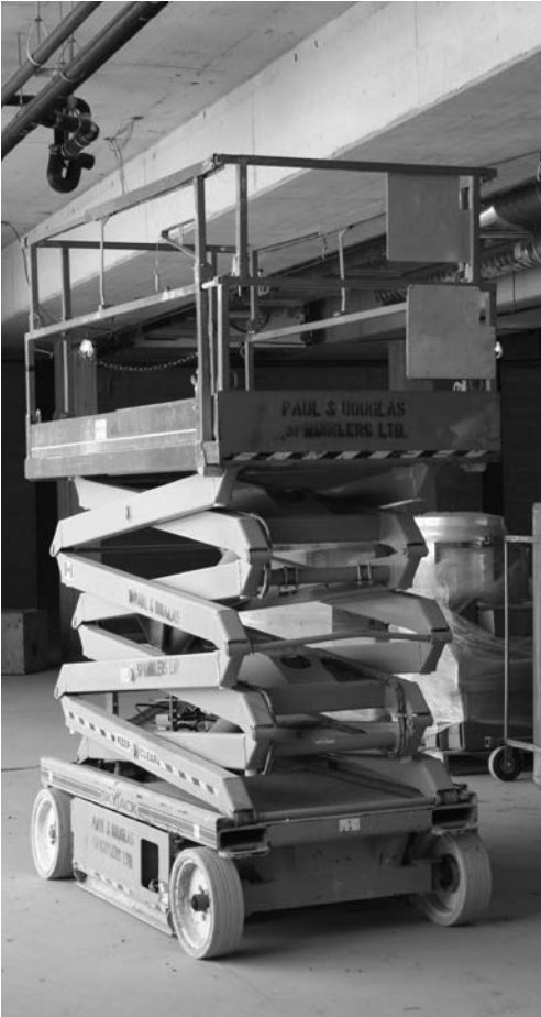
Used to provide temporary access for inaccessible areas at height
